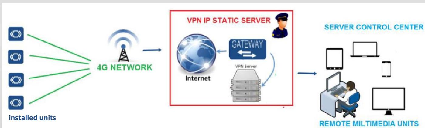
**"CONNECT 4G"** is a special version of "Wave 4G Audio", allowing the connection between two different technologies, infacts can be used stand alone or also to store and forward the audio signal sent by our other audio systems, for example the Puma Plus RF, system based on radio frequency.
