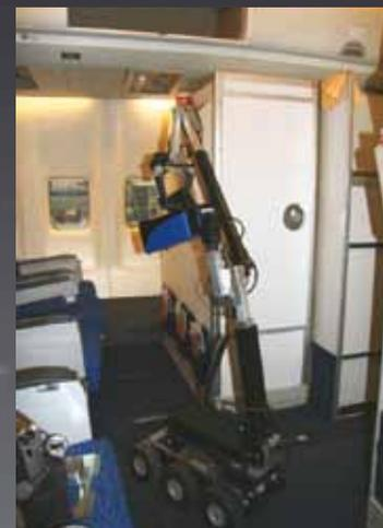
Bomb-squad robot with remotely controlled EXPLONIX in action inside the aircraft
