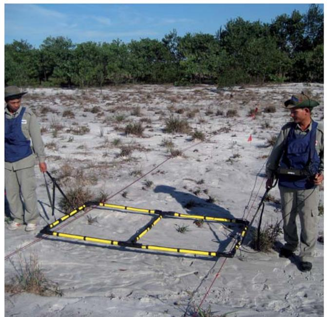
EBINGER UPEX® data logging and detection system
