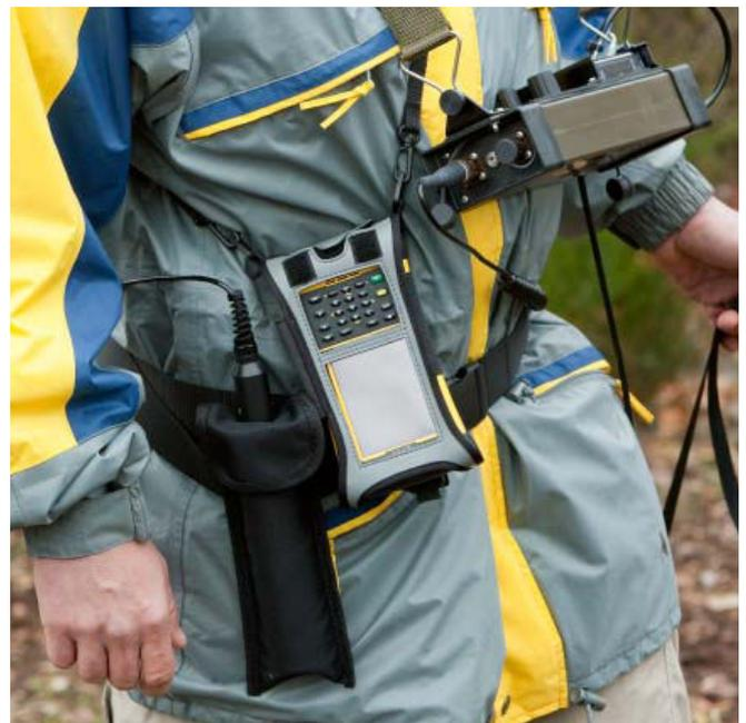
UPEX® 740 M device electronics and EPAD® data logger
