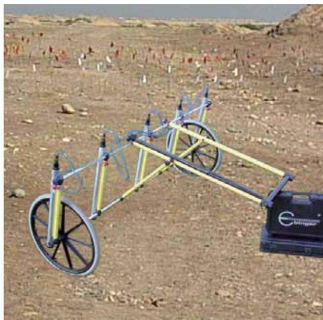
EBINGER MAGNEX® 5-channels magnetic locator system
