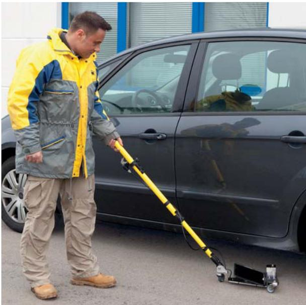
**Under-vehicle search mirror for efficiently inspecting the underside of vehicles**
