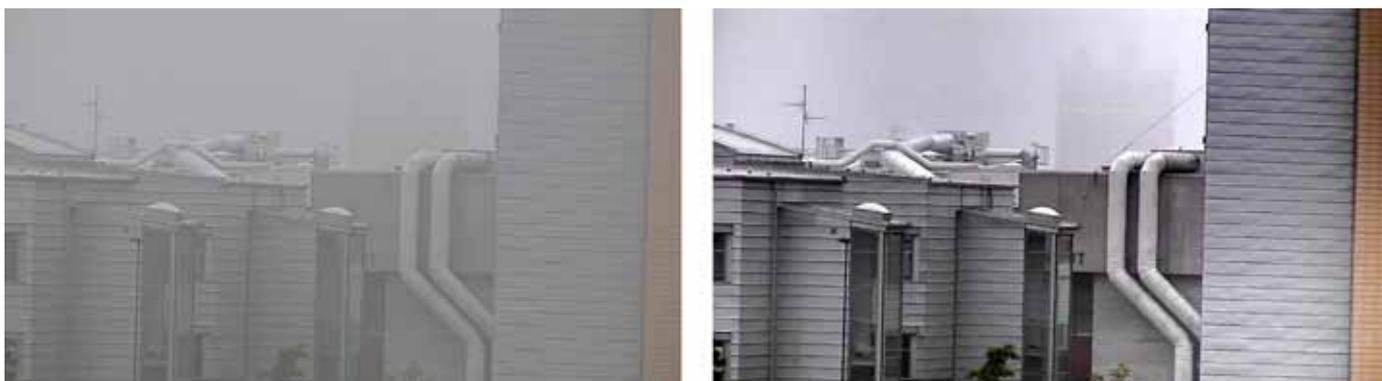
Images from AXIS Q6044-E: at left, without automatic defog; at right, with automatic defog activated.
