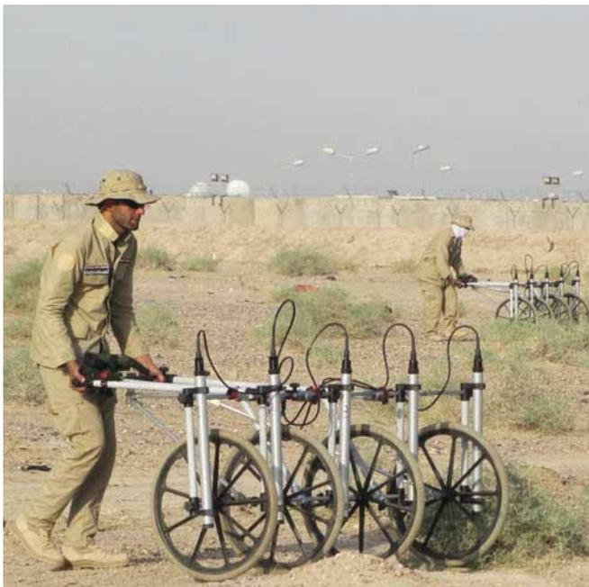
MAGNEX® 120 LW Three-channel-array system
