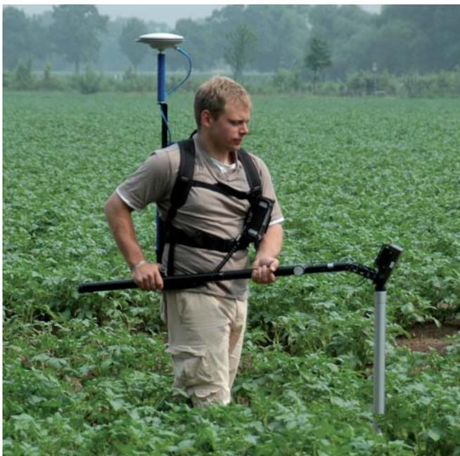
EBINGER MAGNEX® with EPAD® data logger and OMNISTAR DGPS system
