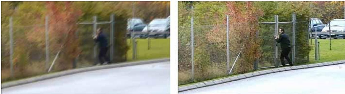
Under vibrating conditions: at left, image without EIS; at right, a snapshot from a vibrating AXIS Q6044-E with EIS activated.
