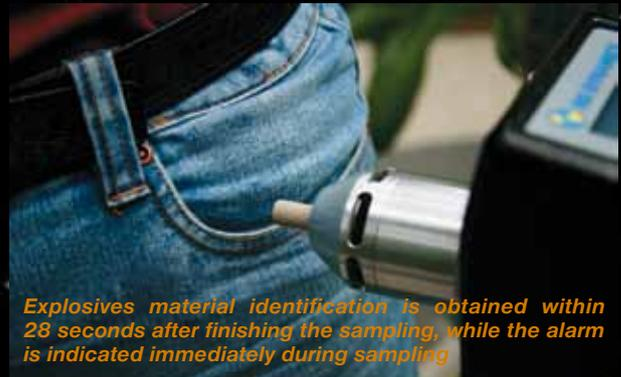
*Explosives material identification is obtained within 28 seconds after finishing the sampling, while the alarm is indicated immediately during sampling*
