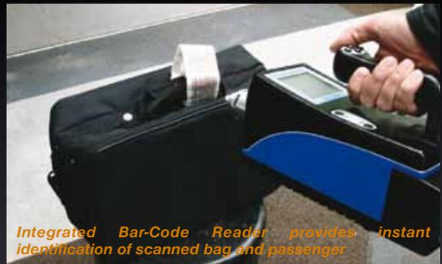
*Integrated Bar-Code Reader provides instant identification of scanned bag and passenger*
