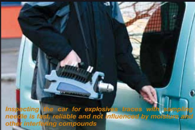
Inspecting the car for explosives traces with sampling needle is fast, reliable and not influenced by moisture and other interfering compounds
